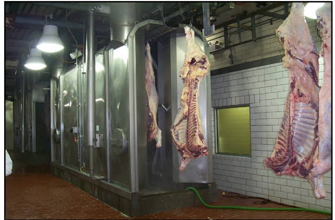
A hot water cabinet is used to pasteurize carcasses before processing.
