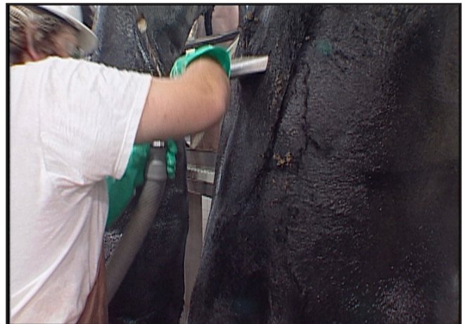
A worker applies a steam vacuum to areas of visible contamination that may contain bacteria
